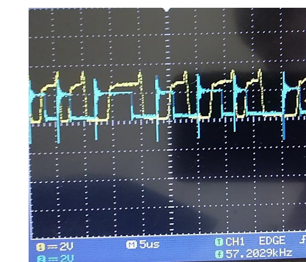
Figure 10: The Results From the TX Pin (Blue) Versus the RX Pin (Yellow)
